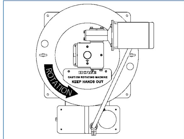
The Drive Motor and Speed Reducer should be placed in the orientation shown above.
