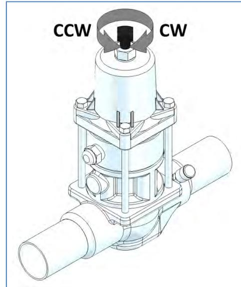
To increase the pressure setting, rotate clockwise.
