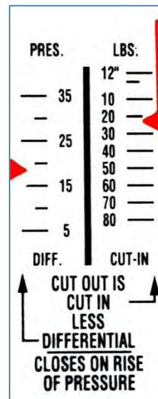
The left side of the control indicates pressure differential for Cut-Out (compressor off) and the right side indicates pressure for Cut-In (compressor on).
