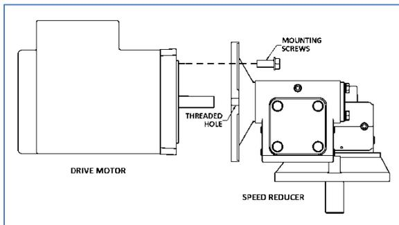
Drive Motors may provide a good deal of resistance when being removed. There are (2) threaded holes on the face of the Speed Reducer
