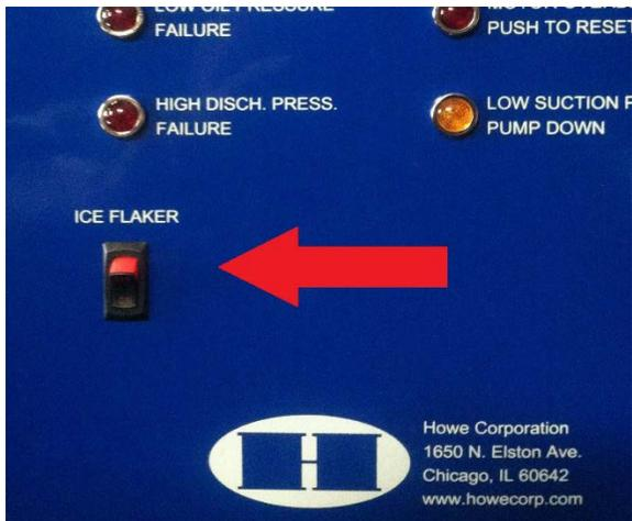
1. Turn the Power Switch “Off” at the Ice Flaker Control Panel.
