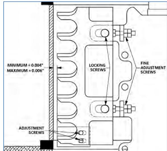
A set of feeler gauges should be used to determine the distance between the Ice Blade and the Evaporator.
