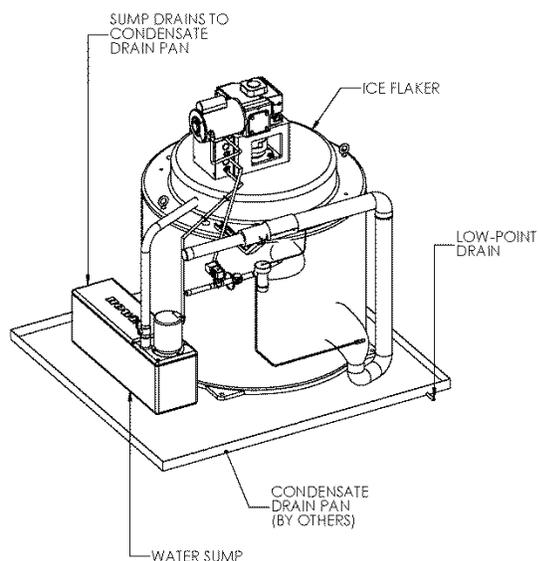
The Drain Water Piping figure above illustrates the location of the low-point drain, which is to be piped to the nearest sewer hub or trench drain.
