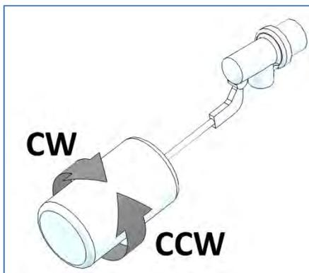
Adjust the water level by rotating the float end of the Float Valve. Rotate clockwise to raise the water level and counterclockwise to lower the water level.
