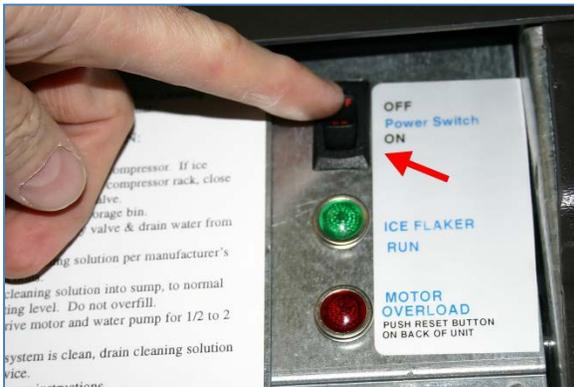
1. Turn the Power Switch “Off” at the Ice Flaker Control Panel.
