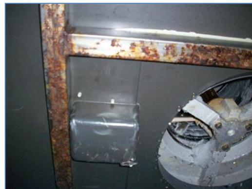
If not removed from water, chlorine mixes with moisture in the Ice Flaker and Ice bin to form a mild hydrochloric acid. This acid can cause surface rust to form on stainless steel surfaces in one to two years.
