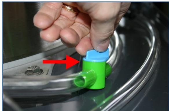
5. Open Ice Flaker Stop Valve to allow water to exit from Water Sump. Afterwards close Stop Valve to prevent loss of solution.
