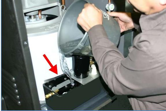
7. Pour cleaning solution into Water Sump to a level just below the side opening.
