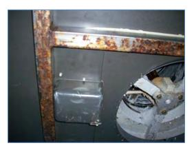
If not removed from water, chlorine mixes with moisture in the Ice Flaker and Ice bin to form a mild hydrochloric acid. This acid can cause surface rust to form on stainless steel surfaces in one to two years.
