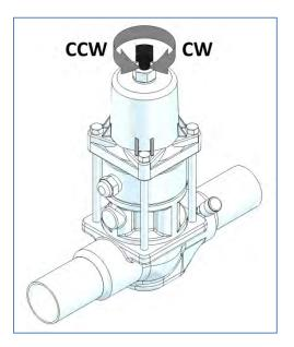
To increase the pressure setting, rotate clockwise.
