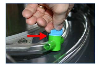
Open Ice Flaker Stop Valve to allow water to exit from Water Sump. Afterwards close Stop Valve to prevent loss of solution.
