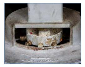
The effects of scale and sediment can be very destructive to the Ice Flaker.
