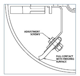
With normal usage, the Squeegee can wear over time. Worn Squeegees need to be trimmed or replaced.
