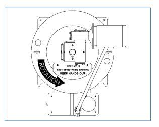
The Drive Motor and Speed Reducer should be placed in the orientation shown above.
