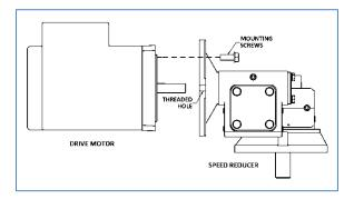
Drive Motors may provide a good deal of resistance when being removed. There are (2) threaded holes on the face of the Speed Reducer in which the mounting screws can be inserted to help push the Drive Motor away. One motor power lead for the Drive Motor should pass through the Overload Sensing Coil on the Control Module (1) time.(230/1/60 panels only, 3 phase motors have electronic overload sensing devices).
