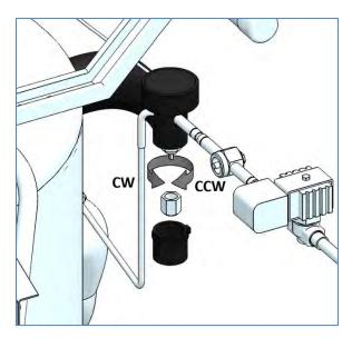
Superheat is not a reliable method of adjusting TXV on Ice Flaker. TXV must be adjusted while visually inspecting the Evaporator's freezing surface.
