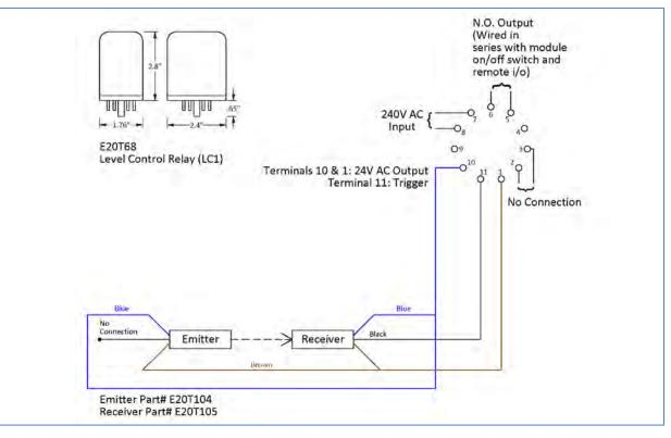
The Photoelectric sensors, or Photo Eyes, shoot an infrared beam across the opening of the Ice Flaker.
