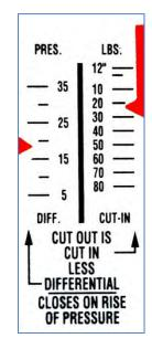
The left side of the control indicates pressure differential for Cut-Out (compressor off) and the right side indicates pressure for Cut-In (compressor on).
