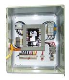
Electric control panel is shipped loose, to be field mounted & wired. Includes drive motor contactor, solid state overload device for drive motor & off delay circuit for optimum protection.
