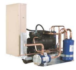
Semi Hermetic water cooled R-404A condensing units for shipboard installation. Condenser fitted with Cupro-nickel tubes for seawater.
